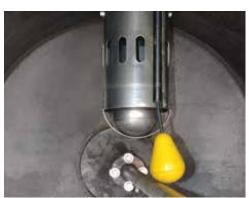
**DUAL TANK SHUT-OFF SYSTEM.**Reduces the rick of material entering the blower - in turn, adding greater longevity to your system.
